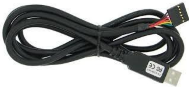
Figure 3 FTDI cable showing the two ends
