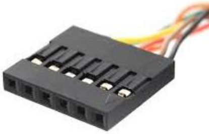
Figure 4 Head of FTDI Cable, which connects to the Mote
